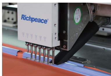
Side-discharged Punching Needles
